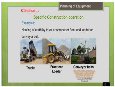
So, similarly, another example on hauling of earth as I told you the hauling of earth or you can either go for a truck, even the scraper what we saw in the earlier slide the scraper also can is good for a hauling distance up to 1000 meter it is economical. So, even you can go for a scraper for hauling of earth. So, there are different hauling machines available you can either go for a truck, which is the best hauling equipment or you can go for a front end loader.
