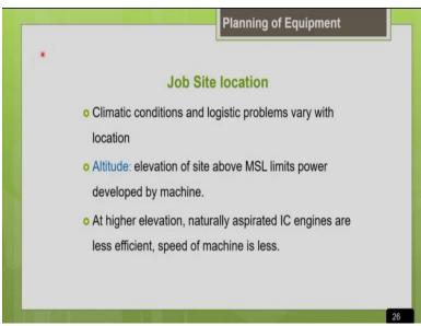
So, far we discuss about the job site conditions now we are going to see how the job site location is going to affect the selection of the machine. So, that is basically it is going to affect the climatic conditions of the place and other logistic problems involved with the mobilization of the equipment at the particular site. So, all these things are dependent upon your job site location.
