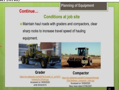
Another important guideline which we should keep in mind is we should always maintain the haul roads, there are so, many equipment's to maintain the haul road, like either you can go for a grader or you can go for a compactor. So, you should maintain the haul roads clear all the short rocks so, that you can increase the travel speed of your machine. So, if you can increase the travel speed of your machine, the cycle time of the machine will be reduced.
