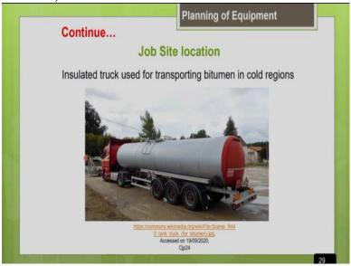
So, this picture shows you an insulated truck which is used for transporting the bitumen. So, this will help you to maintain the temperature of the bitumen as I told you, the working temperature of the bitumen is very critical. So, you have to maintain it at temperature similarly, even your ready mix concrete trucks you can go for insulated RMC trucks particularly in the cold weather countries in order to maintain the working temperature.
