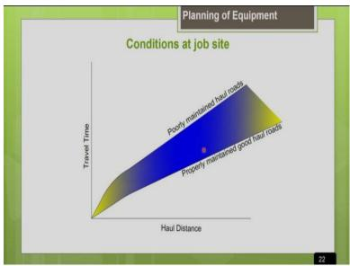
So, this graph shows you the difference in the travel time of a vehicle which is running over a poorly maintained haul road and another vehicle running on a properly maintained haul road you can see there is a significant reduction in the travel time of the machine. So, this will definitely influence or affect the productivity of the machine and the cost of the project.
